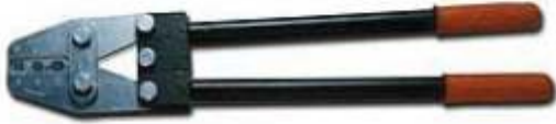
H - 50 ( Dieless ) Crimping Capacity : for Cu. & Al. crimping socket : 25mm 2 , 35mm 2 & 50mm 2 for Ring Type : 16mm 2 , 25mm 2 & 35mm 2
