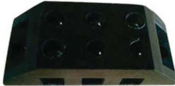
Single Way Earth Bar Product Code:-DEEB-02 Current Rating 32 Amps. Material :- Base-Backalite. Terminal-M.S zinc plated.
